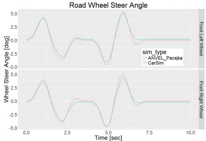
**Figure 3:** Wheel steer angle for both ANVEL and CarSim models in the double lane change test.
