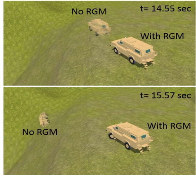
**Figure 18:** Sample simulation screenshots showing that the test vehicle with RGM successfully stopped in front of a road-side slope, while the baseline vehicle fell down the slope.
