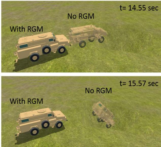
**Figure 16:** Sample simulation screenshots showing that the test vehicle with RGM successfully stopped in front of a pothole, while the baseline vehicle fell in.
