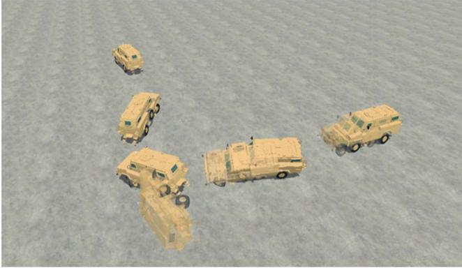
**Figure 20:** Sample screenshots showing the difference between the baseline vehicle and the one with RGM. Solid images represent the vehicle with RGM; opaque images are the baseline vehicle. The forward speed was 8 m/s for both vehicles in this test.
